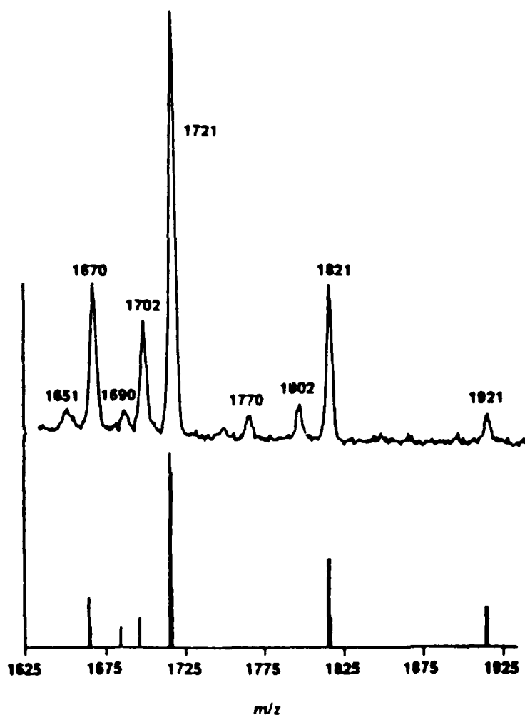
Fig. 6. Comparison of the ion trap spectrum of Ultramark™-1621 with a standard EI mass spectrum [50].
